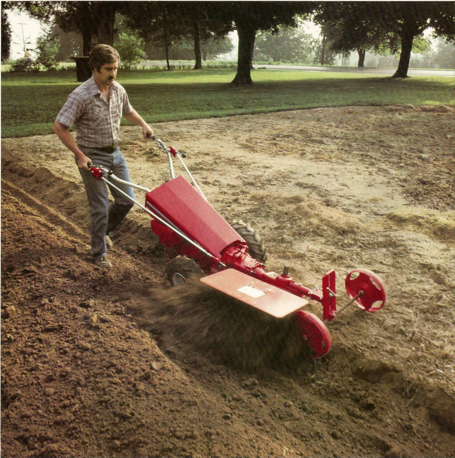
Above: 5200, 8 HP Tractor with High-Speed Rotary Plow. Right: Detail of Rotary Plow.
